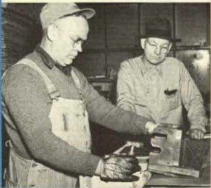
Another item bought outside are these Wheelabrator wheel spacers being checked in a gauge by Bill Stickle . This gauge as are many other tools used by the inspectors, was designed and built in our tool room for our own particular work.
