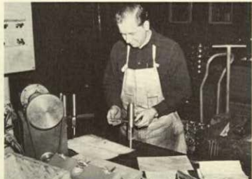
Wheelabrator hubs are an important part of the heart of the Wheelabrator machine. Marion Daxow is performing one of the three inspections on these hubs; testing them on this machine for "run out". The dials show whether the hub is true or not.
