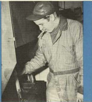
Dick Bidlack is dipping parts into a rubber-like plastic to protect the threads. A dipped part can be roughly handled in shipping or erection without injury.
