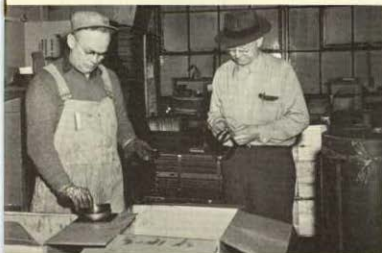
Dick Bidlack is dipping parts into a rubber-like plastic to protect the threads. A dipped part can be roughly handled in shipping or erection without injury.
